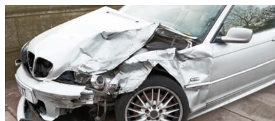
Sections of a car are designed to crumple in an accident.
