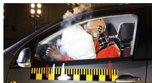
Crash detection, inflation and deflation of the airbag (to allow the driver to see again) must all take place in less time than it takes you to blink!
